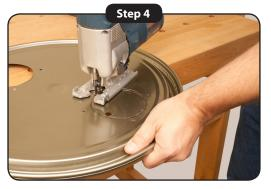
With a jig saw or any suitable cutting tool, cut the holes out of your barrel lid. Note: On some lids it may be easier to drill a pilot hole to create a better starting point as shown above.
