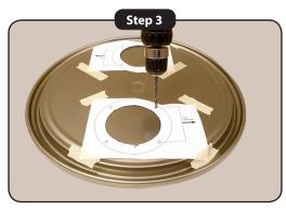
With the templates still taped to the lid, drill the four holes on both template drawings. Once holes are drilled remove the templates.
