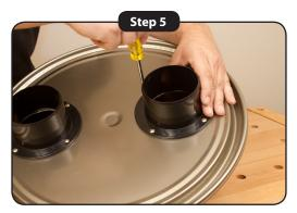
Secure the flanges and the ports with the nuts and bolts that are provided. Be sure the ports are facing in opposite directions as shown in the Step 6 diagram below.
